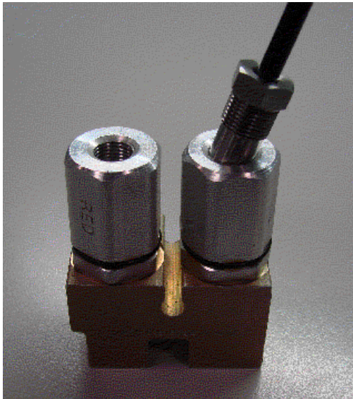
Auto-Drive Fitting and tube incorrectly aligned
