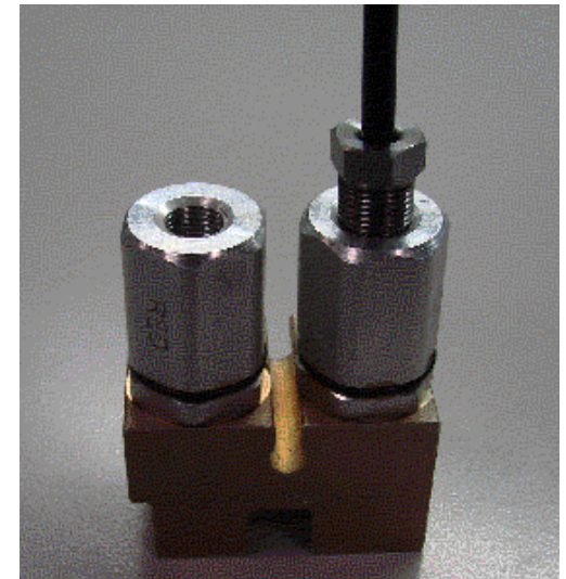
Auto-Drive Fitting correctly aligned and assembled
